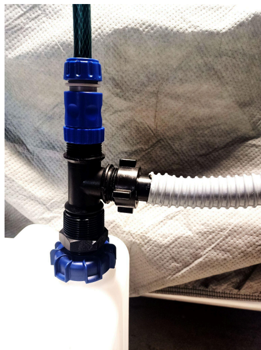
Waste connection using threaded tee connector incorporating vent hose.
