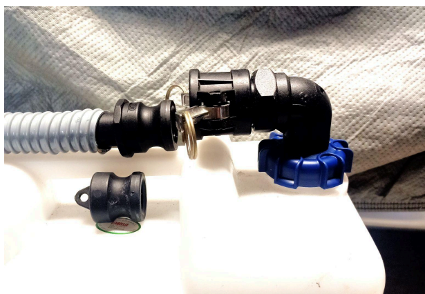
Example of waste connections incorporating clip, camlock fittings with male hose fitting and plug to seal.
